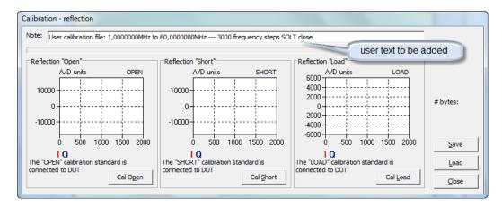
In Reflection mode, three calibrations should be done. ""Open", "Short" and "Load". A describing text for this calibration is shown in the top "Note:" The program will automatically put the calibration range and the
